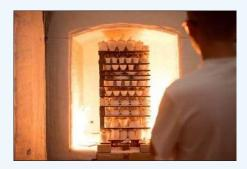
Alumina ceramic solid rods serve as crucial support components and thermal insulation spacers in hightemperature industrial furnaces and kilns, withstanding extreme temperatures up to 1730° C.
